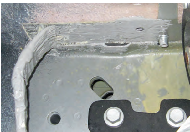
Figure 14: Applying Rust-proofing Paint (2).
