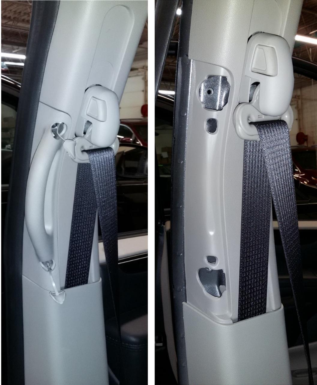
**3) Remove the upper plastic molding from the B-pillar.**
