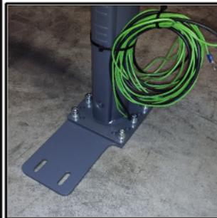
**2) Maneuver eFutureSafe to enable the two slots on the attached Bottom Bracket to fit over the M10 T-bolts as shown.**
