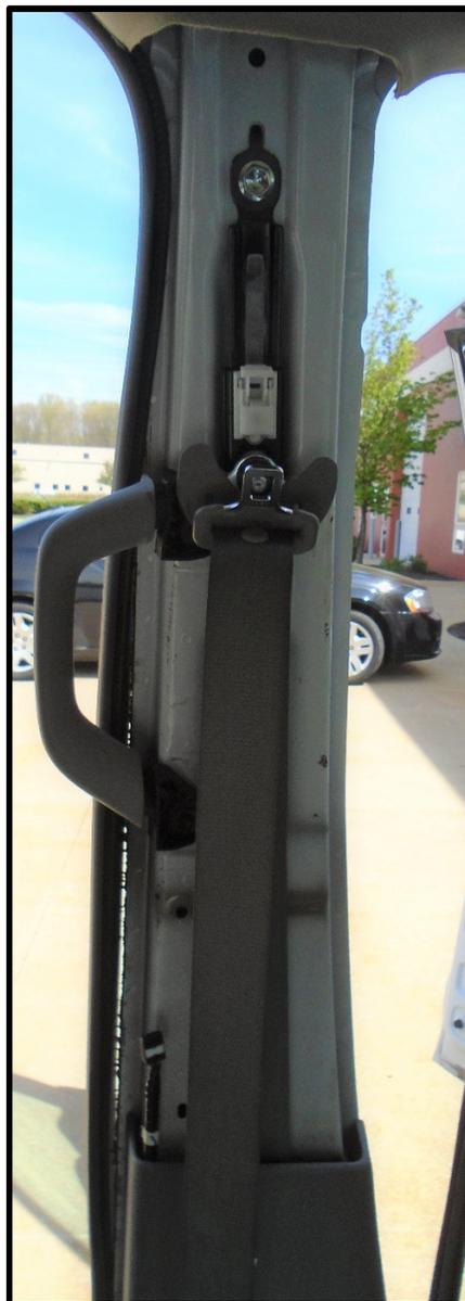
**3) Locate and remove the grab handle on the driver's side B-pillar.**
