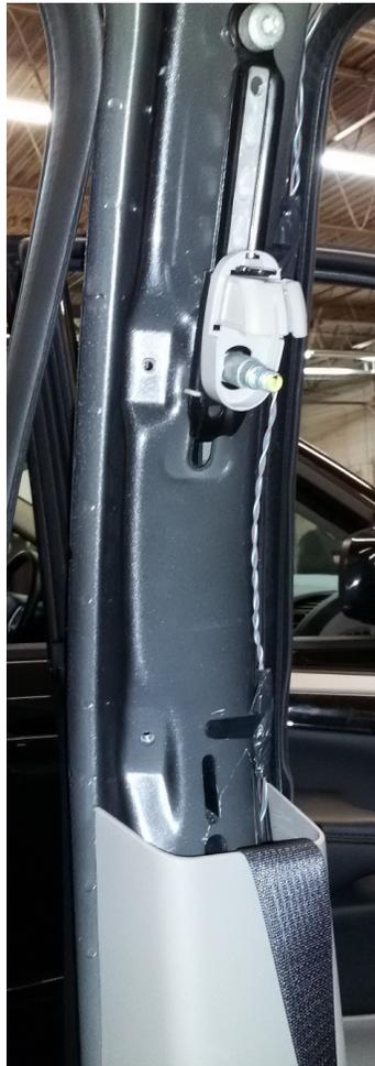
**4) Remove the lock nuts and washers from M10 T-bolts.**
