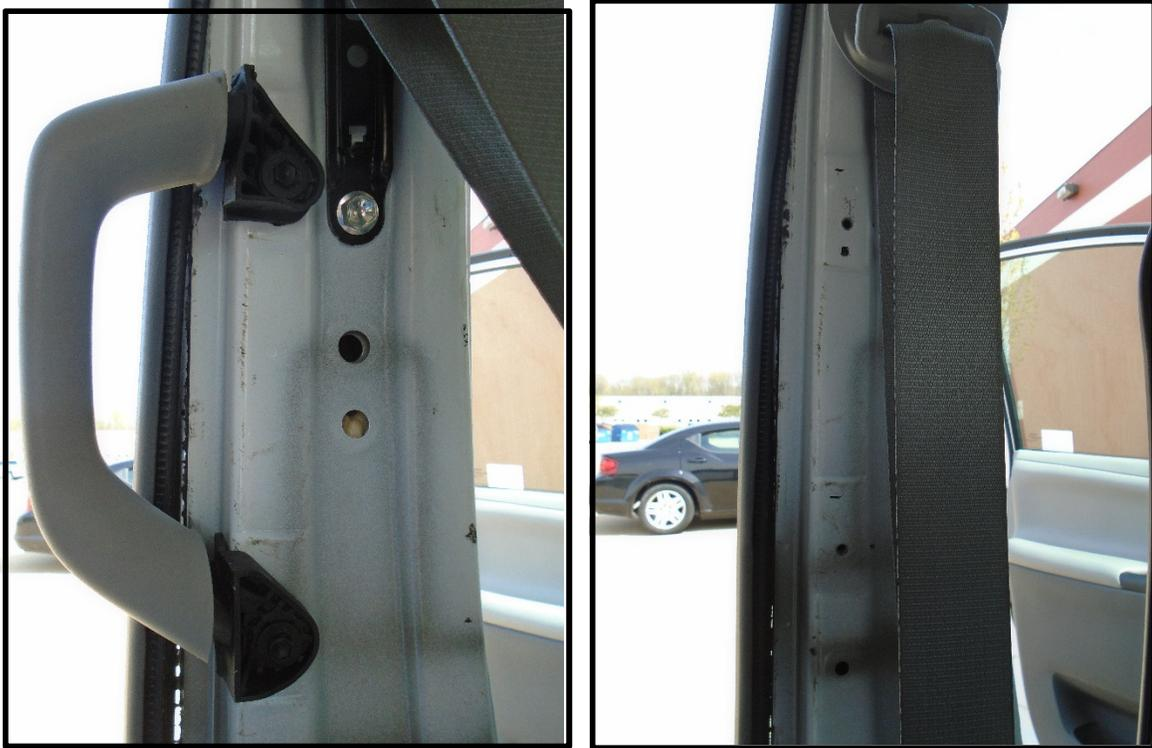
**4) Remove the lock nuts and washers from the M10 T-bolts.****5) Install the two M10 T-bolts into the airline rail located adjacent to the B-pillar.**
